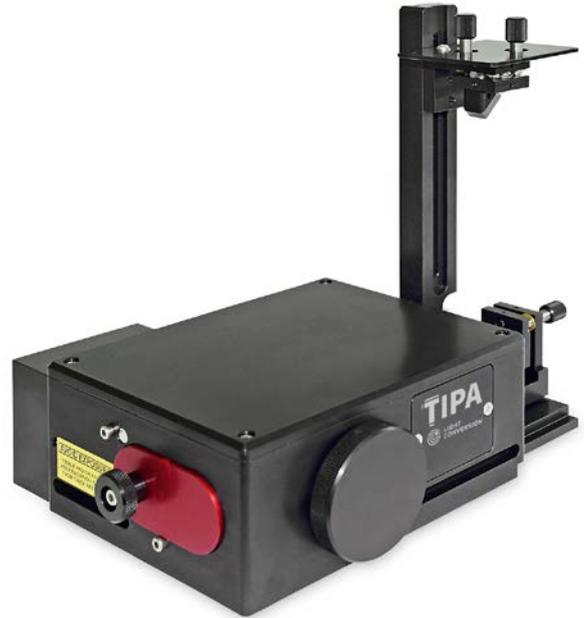
takes place. SH beam's width and tilt in a plane perpendicular to propagation provide information about the pulse duration and pulse front tilt. The SH beam is sampled by the included CCD camera. TiPA comes with a user-friendly software package, which provides on-line monitoring of incoming pulse properties.
