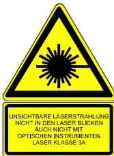
At the point where laser radiation is emitted, a **laser warning sign** must be attached. It provides information about the type of radiation, specific hazards and the degree of protection. The laser warning sign is attached by the OEM customer in accordance to the laser device's classification (⇒ page 6, Classification of laser devices).
