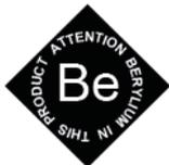
In the high-speed versions of the subsystem the mirrors are made from beryllium. The rating plate indicates if this applies to the present deflection unit (⇒ page 14, Detailed Description). In addition, these deflection units are provided with the adjacent sign. Also note ⇒ page 8, Special hazards caused by mirrors made of beryllium.
