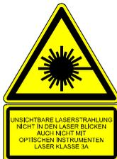
At the point where laser radiation is emitted, a **laser warning sign** must be attached. It provides information about the type of radiation, specific hazards and the degree of protection. The laser warning sign is attached by the OEM customer in accordance with the laser device's classification (⇒ page 5, Classification of laser devices).
