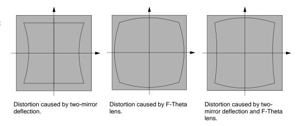
Fig. 4 Example: F-Theta lens for Nd:YAG
