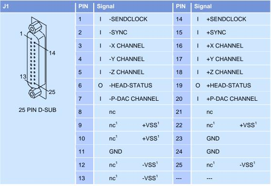
I = Diff. Input, nc = Not connected (not used) O = Diff. Output
